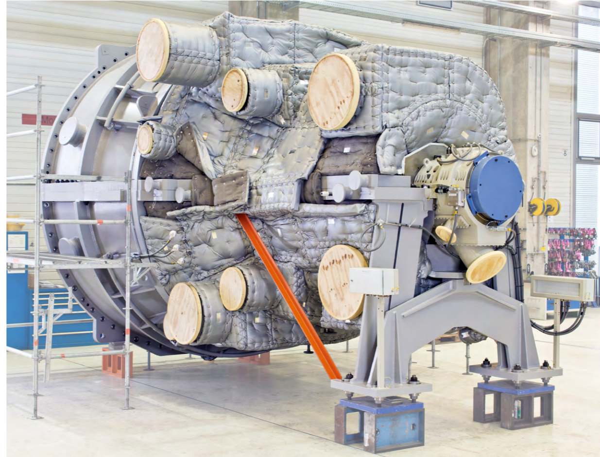
Steam turbine SST-900 for the CSP-plant NOOR III, Morocco
