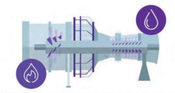
Our dual-fuel capable gas turbines can switch between liquid and gaseous biofuels at any moment – for maximum fuel flexibility.
