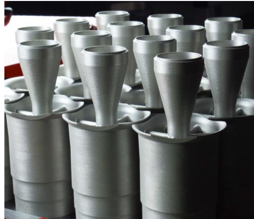
Figure 17: Additive manufactured premixed combustion swirlers for heavy-duty large gas turbines.
