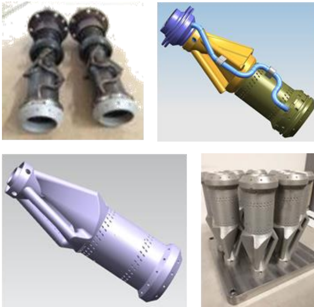
Figure 18: Fuel burner design progressions from welded (top left) to SLM additive manufacturing (bottom right) for 3rd generation DLE burner.
