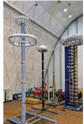
UHV arrester prepared for testing in the HV test laboratory
