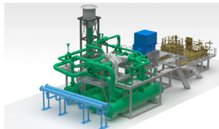
Siemens Energy compressor to be used at Occidental's Direct Air Capture plant.
