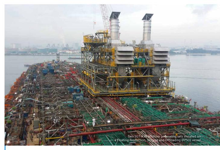
SGT-A35 Aeroderivative gas turbine Power generation: 31.3 – 37.3 MW(e) Mechanical drive: 32.2 – 38.5 MW Based on proven aeroderivative design, the **SGT-A05** gas turbines are flexible, compact and lightweight designs that are ideally suited for decentralized power generation offering high efficiency and fast start-up capabilities.
