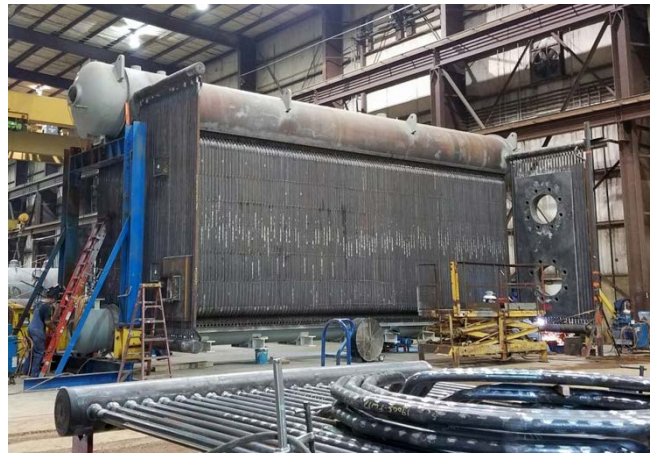
We have package boiler manufacturing experience utilizing a variety of materials and casing construction including internally insulated and lined, refractory lined and membrane wall construction.
