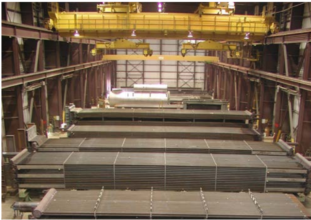
For large frame combined cycles the HRSG pressure parts are manufactured as individual coils (or harps).
