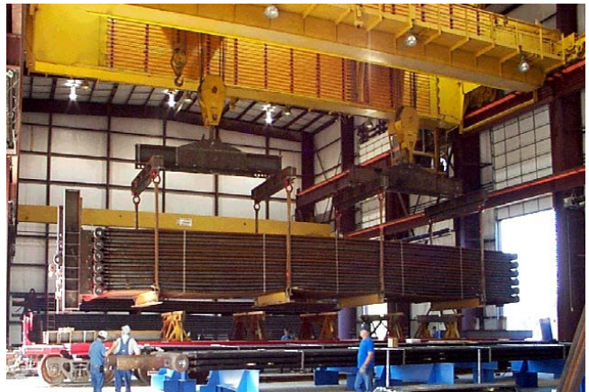
The Chanute facility features 22 overhead cranes with capacities up to 200 tons and 35-foot hook heights.
